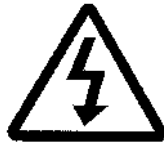
Danger!: High voltage
