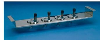
Viscometers such as Cannon-fenske type and Ubbelohde type can be attached and are convenient for measuring kinematic viscosity. (If kinematic viscosity is measured using a BK/BA type water bath, it does not comply with JIS K 2283.)
